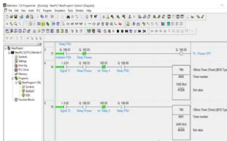
Gambar 3. Diagram Ladder Timer Proses Elktrolisis
